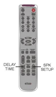
1. Press **SPK SETUP** on the remote control as shown.
